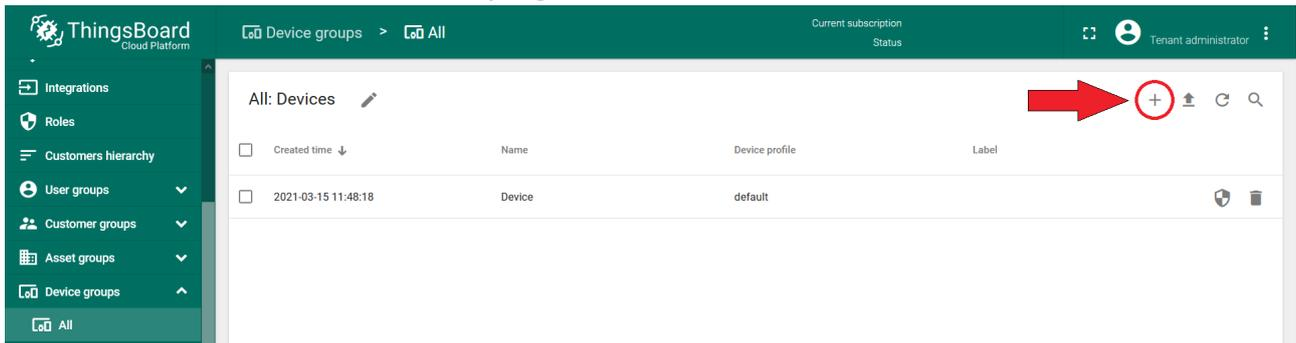
5. Input device name. For example, "My New Device". No other changes are required at this time. Click "Add" to add the device.
