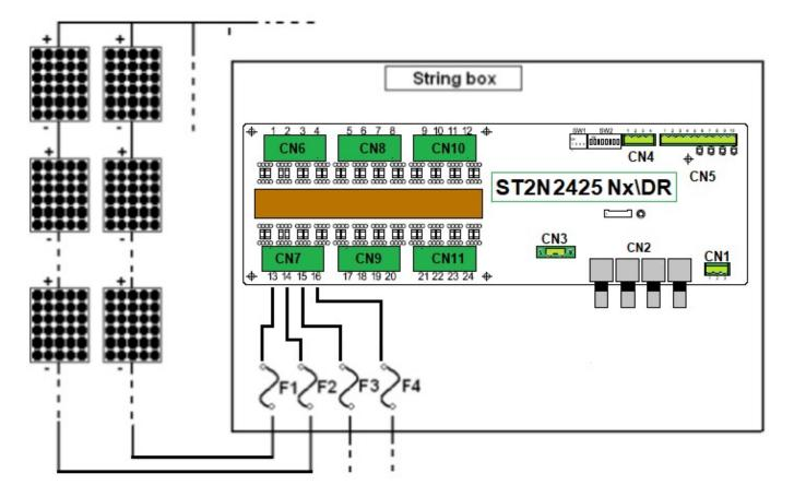
After the strings input connector, on the ST2N board there are two resistors in parallel, they are necessary to detect the current follow :
