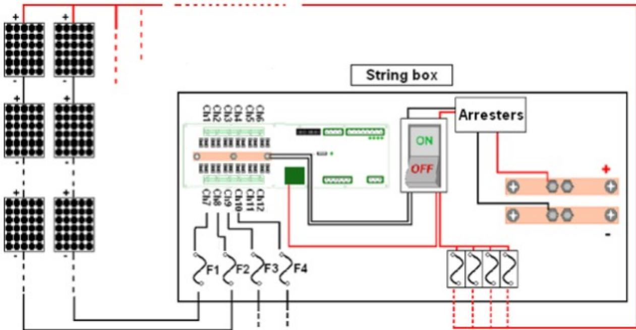
In the following image there are the “ST2N string controller” with all the wiring. Obviously isn't necessary connect all the specified devices, they are indicated to give a connection general idea.
