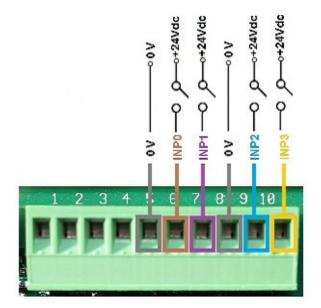
May be necessary connect a probe to a junction box, for example a pyrometer (to know the solar irradiation). To this purpose there are two analog inputs: one which allow to connect a signal which can be from 0 to 20 mA and the other one which allow to connect a signal from 0 to 10 Vdc. The connection is to pin 1, 2, 3 and 4 of terminal block CN5. On register 30042 and 30043
