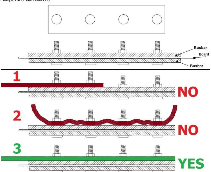
If it is necessary to "extend" the busbar, the following <u>fundamental</u> rules must be followed :
