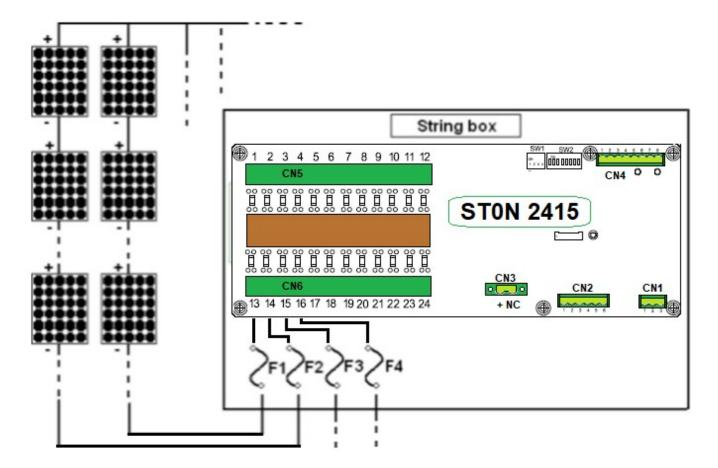
After the strings input connector, on the STON board there is a resistor, it is necessary to detect the current follow :
