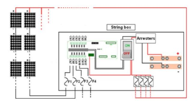
In the following image there are the "STON string controller" with all the wiring. Obviously isn't necessary connect all the specified devices, they are indicated to give a connection general idea.
