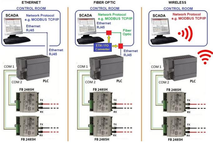
Typically the PLC communicates via Modbus TCP / IP protocol with the SCADA in the control room with Ethernet or fiber optic or wireless connection.
