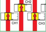
IF YOU USE THE "-" [NEGATIVE] CABLE Insert the cable from the TOP to the BOTTOM :
