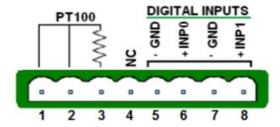
Is possible connect one PT100 to read the external temperature. The PT100 could be 2 or 3 wires, it will be connected as shown in the figure above to terminal block CN4. You can find this temperature on register 30044.
