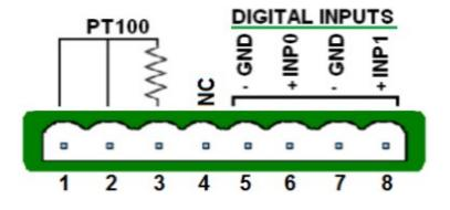
Is possible connect one PT100 to read the external temperature. The PT100 could be 2 or 3 wires, it will be connected as shown in the figure above to terminal block CN4. You can find this temperature on register 30044.
