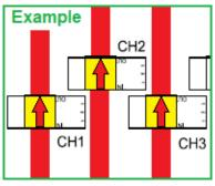
IF YOU USE THE "-" [NEGATIVE] CABLE Insert the cable from the TOP to the BOTTOM :
