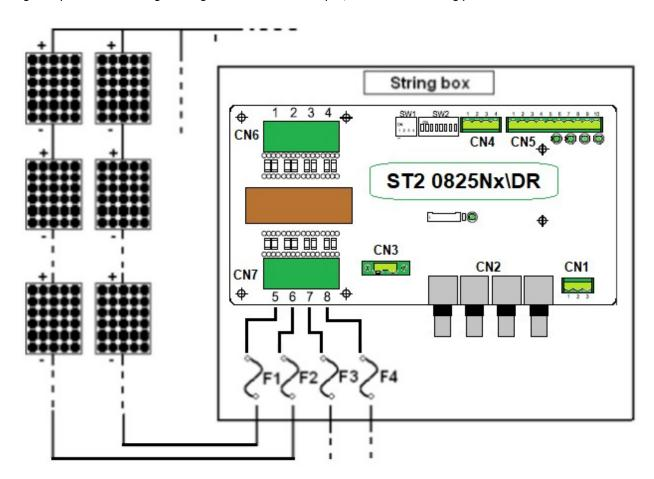
After the strings input connector, on the ST2 board there are two resistors in parallel, they are necessary to detect the current follow:
