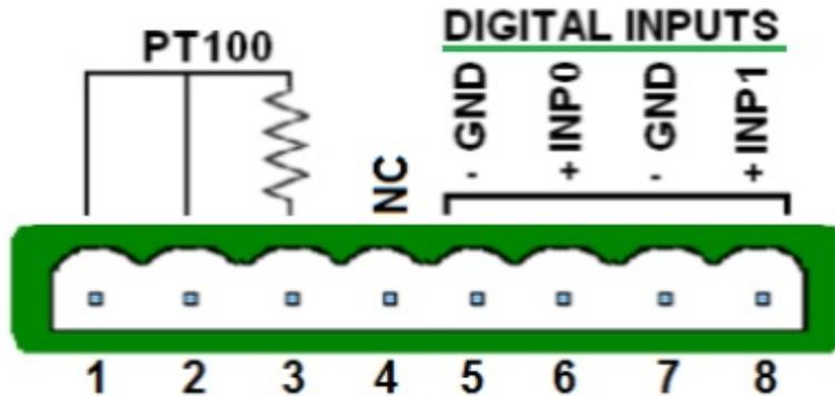
Is possible connect one PT100 to read the external temperature. The PT100 could be 2 or 3 wires, it will be connected as shown in the figure above to terminal block CN4. You can find this temperature on register DATA.30044.
