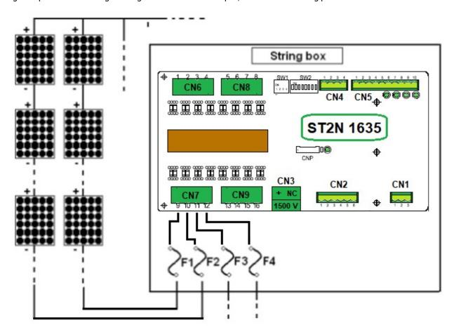
After the strings input connector, on the ST2N board there are two resistors in parallel, they are necessary to detect the current follow:
