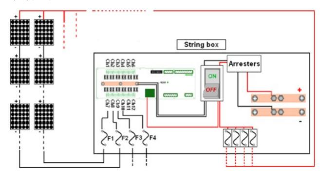
In the following image there are the "ST2N string controller" with all the wiring. Obviously isn't necessary connect all the specified devices, they are indicated to give a connection general idea.
