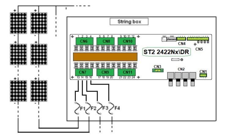
After the strings input connector, on the ST2 board there are two resistors in parallel, they are necessary to detect the current follow :
