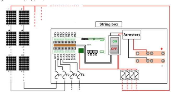
In the following image there are the "ST2 string controller" with all the wiring. Obviously isn't necessary connect all the specified devices, they are indicated to give a connection general idea.
