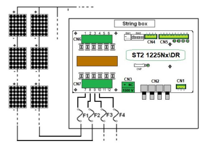
After the strings input connector, on the ST2 board there are two resistors in parallel, they are necessary to detect the current follow :
