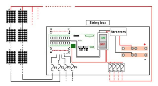
In the following image there are the "STON string controller" with all the wiring. Obviously isn't necessary connect all the specified devices, they are indicated to give a connection general idea.
