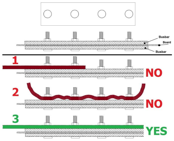
If it is necessary to "extend" the busbar, the following fundamental rules must be followed:
